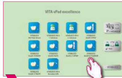
3 Press on the desktop and hold until the desktop editing menu appears.
