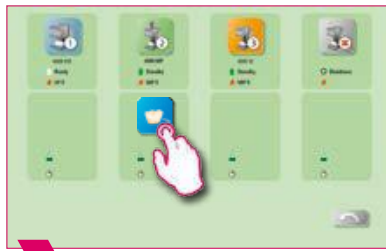
2 Multifurnace: Press and hold the firing program button to move it if you want to use another firing device.
