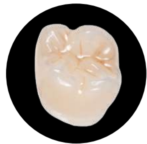
Stained crown prior to wear test
