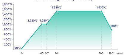
Fast Sintering Parameters (1-3 Units)
